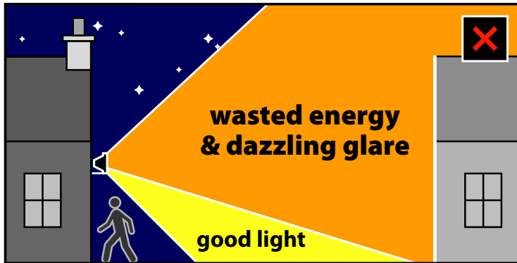
BADLY AIMED 500W HALOGEN FLOODLIGHT
